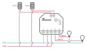
② Connect SPDT switches in the edge mode to reach double two-way control:
