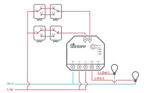
3 Connect dry contact sensors in the following mode:
