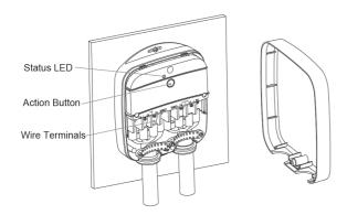
Action button: Used for Heavy Duty Smart Switch Z-Wave network inclusion and exclusion and to manually turn on or off.
